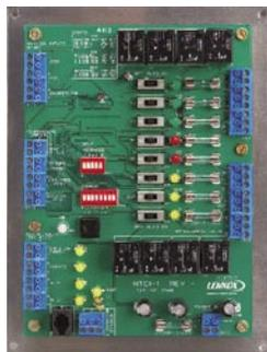
Zone Controllers and Sensors provide basic control at each zone
